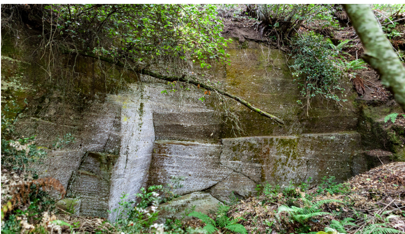
Fig. 1 and 2. Author: Elena Lavellés. Photographs of the quarries of Tusculum. The city of Tusculum was one of the largest and oldest in Italy. In its quarries you can still see the marks of the tools left more than two thousand years ago by the workers when extracting the stone blocks.
