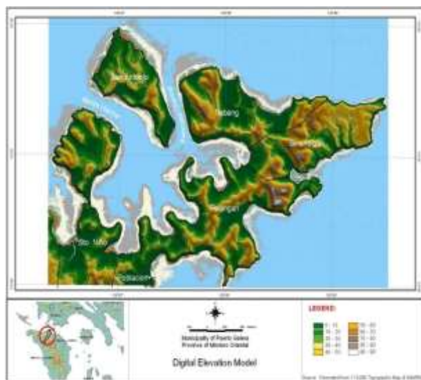
Figure 8 Digital Elevation Model (DEM) extracted from the 1:10,000 topographic map of NAMRIA
